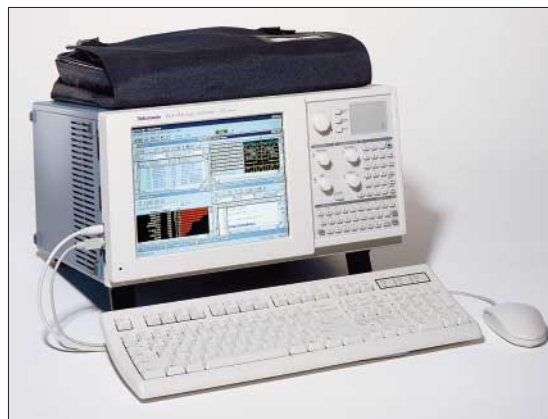
Figure 20. The Tektronix TLA 700 Series Logic Analyzer's 3.4 Gb/s acquisition data bandwidth surpasses Rambus data rate requirements of 1.6 Gb/s.
