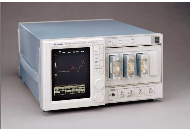
Figure 5. Typical High-Resolution TDR (Tektronix 11801C with SD-24 TDR Sampling Head).
